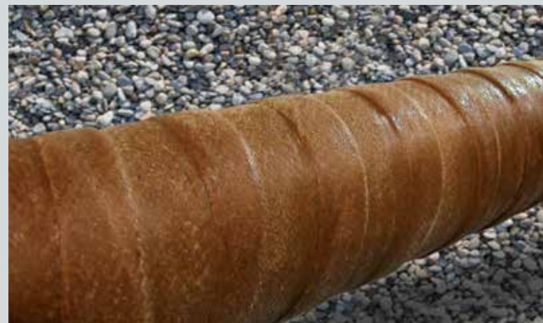
Trenton's Wax-Tape® HT-3000 high-temperature anticorrosion wrap will perform effectively at continuous operating temperatures up to 230 °F (110 °C). When used aboveground, an outerwrap such as Trenton's MCO® 110 outerwrap is recommended.
